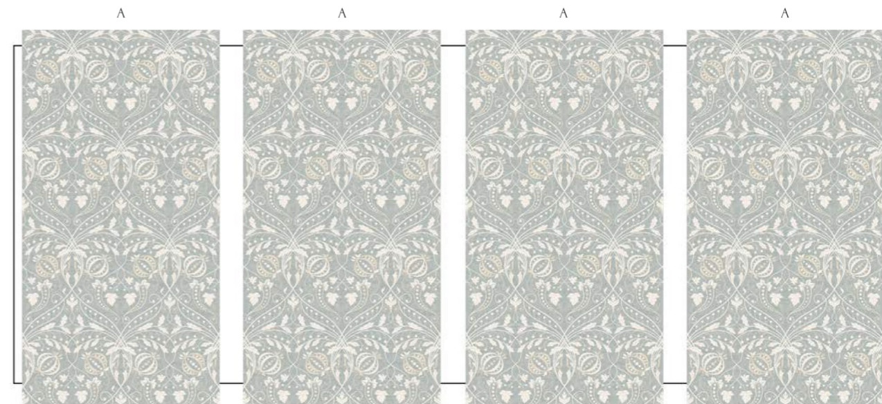
CHATEAU is an example of a straight repeat where all panels will be identical.
